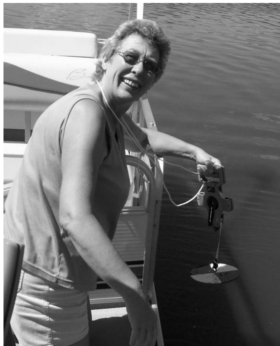
CLMP Volunteer Nancy Beckwith demonstrates the use of a Secchi disk, a simple tool for measuring water transparency. Diminished water transparency is a possible indicator of eutrophication. (MiCorps photo by Jo Latimore)
