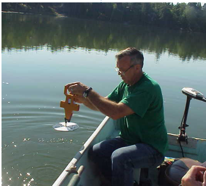
A CLMP volunteer uses a Secchi disk to measure the depth of light penetration in a lake. Photo: MLSA
