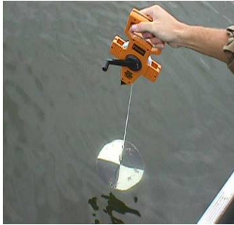
The Secchi disk is named after Pietro Angelo Secchi, who in 1865 used a white disk to take transparency measurements in the Mediterranean Sea (credit: MiCorps).
