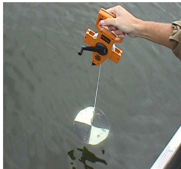
The standard Secchi disk used in the CLMP. Credit: Ralph Bednarz, EGLE
