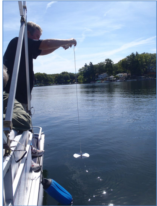
A CLMP volunteer on White Lake (Oakland County) uses a Secchi disk to measure water transparency, a standard approach to assessing lake productivity. (MiCorps photo by Angela De Palma-Dow).
