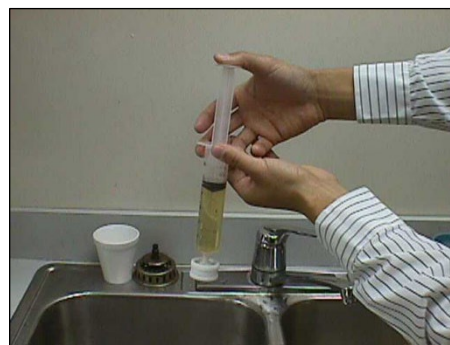
F7. Adjust pressure to achieve steady drops (drop drop drop drop)
