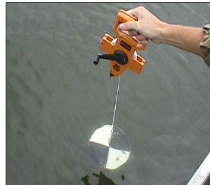
The Secchi disk is named after Pietro Angelo Secchi, who in 1865 used a white disk to take transparency measurements in the Mediterranean Sea.
