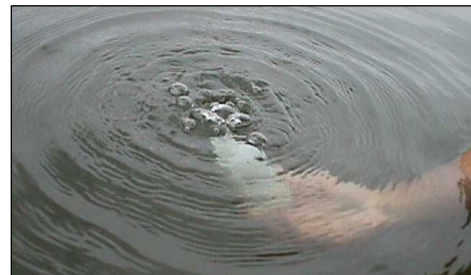
A phosphorus sample is collected by lowering the bottle upside down 1-2 feet below the surface, then pointing the bottle up, allowing the bottle to fill.
