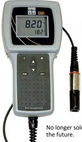
DO/Temperature Equipment YSI Oxygen Meter (550A or Pro-20)
